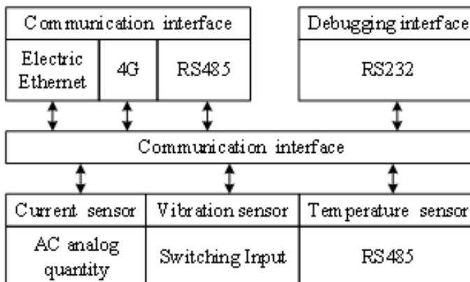
Figure 4. Software architecture of cable edge intelligent terminal
