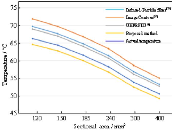
Table 5. Temperature measurement errors of different methods under different currents
