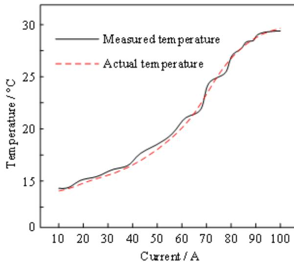
Table 2. Temperature measurement error of power cables under different currents
