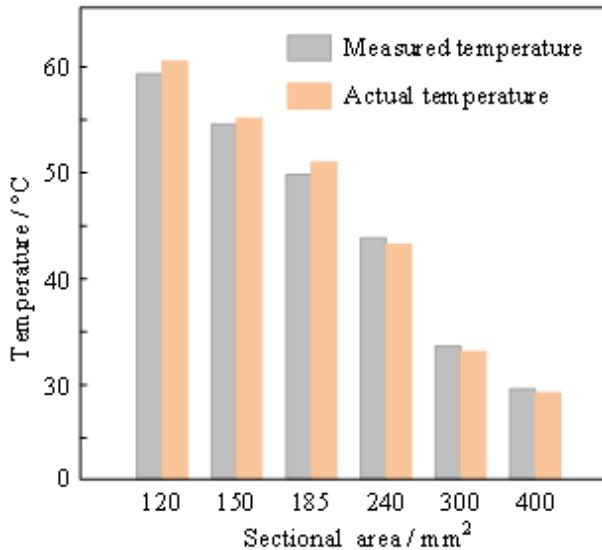
Table 3. Temperature measurement error of power cables with different sectional areas
