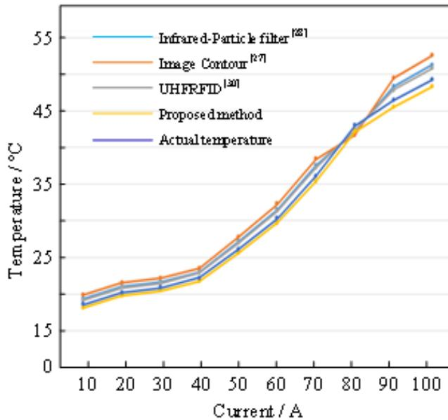
Table 4. Temperature measurement errors of different methods under different currents
