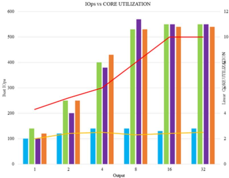
The remote storage engine system needs to use RDMA and SPDK technology to accelerate and reduce network latency. As shown in Figure 3, the performance of the I/O mode utilizing SPDK is compared and analyzed against the normal Linux kernel on the Optane SSD DC P4800X disk. It is evident that as the queue depth (qp) increases, SPDK has an obvious acceleration effect on high-performance disk devices, reaching 500k IOPS.
