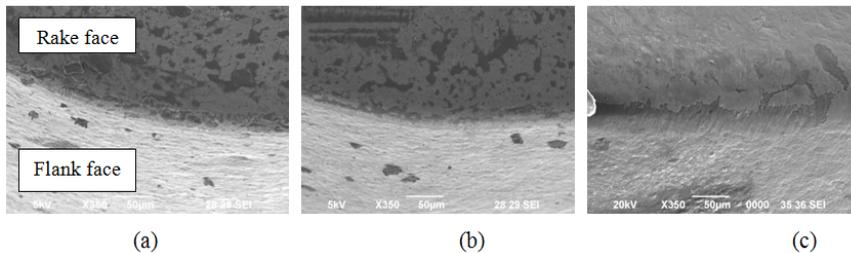
Figure 12. Chip microgram during the application of (a) coconut oil-based cutting fluid (b) raw coconut oil (c) mineral oil-based cutting fluid (V=80 m/min, f=1 mm/rev, d=1.25 mm) (Magnification 100 X)
