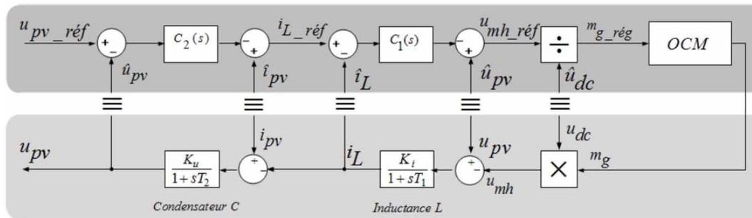
Figure 5. Block diagram of the grid side
